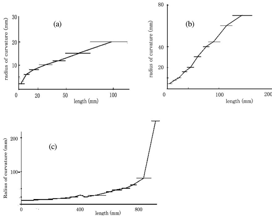
Fig. 2. The measured  $R(l)$  curves for (a) the Archimedean, (b) the logarithmic and (c) the Comu's (hyperbolic) spirals. The horizontal bars show the lengths of arcs used in the measurement.
