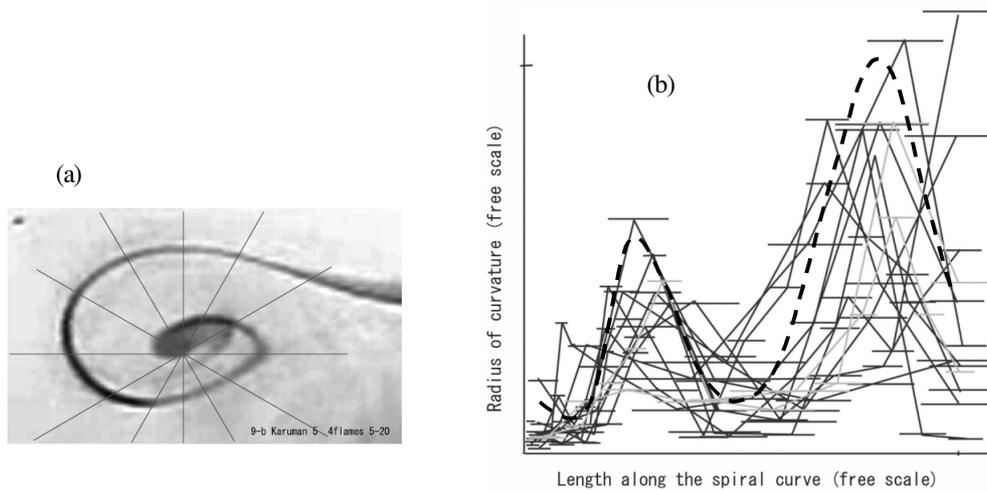
Fig. 4. (a) A visualized vortex, (b)  $R(l)$  curves for visualized vortices behind a moving cylinder, where two gray curves are obtained from the vortex shapes visualized by TANEDA (1988). The dashed line indicates a common feature of these curves.
