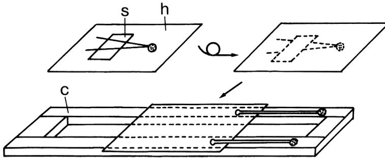
Fig. 2. Illustrations of the holder (h) and the perfusion chamber (c). The skin preparation (s) was fixed on the holder so that the skin surface (epidermis side) came to contact with the coverslip. The holder was then turned over and placed on the chamber.
