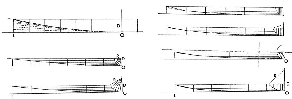
Fig. 4. Various Drawing Procedures for Curves of Eaves.
