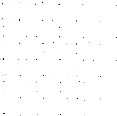
Fig. 3 b Diffraction pattern of octagonal lattice
